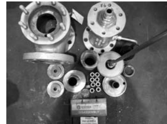
Valve Dis-Assembly
